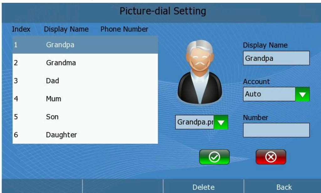
**Instruction:** This feature allows user to call out directly by touching the six icons of the picture dial screen after setting the corresponding values of the icon. You can enter the Picture Dial configure screen by the path listed above. For example you can configure the fifth icon, "Display Name": AA, the current "Account": auto, the dial out number: 1111, the default icon: son, and save the settings. The capture screen shows the result with the settings.
