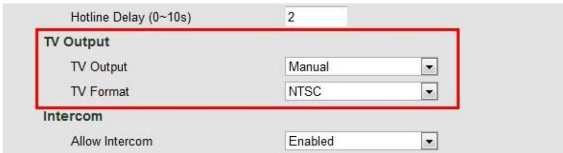
**Instruction:** The "TV Output" is used to configure the video format of TV Output and configure the mode of outputting video call to the external equipment, by Manual or auto. If "TV Output" is auto mode, the video will be outputted to the external equipment automatically when the phone starts a video call. If "TV Output" is manual mode, you have to click "TV OutPut" to output the video to the external equipment manually.
